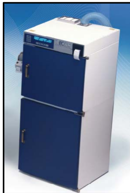
NHSRC's Laboratory EtO sterilizer
